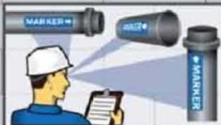
Label placement in relation to point of normal approach
